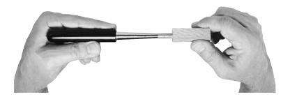
This tool can be used to aid in the insertion and gluing of pen tubes between 7mm and 11mm. Simply place the pen tube over the end of the tool and cover with your choice of glue. Be sure to cover the entire surface, leaving no bare spots.
