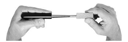
This tool can be used to aid in the insertion and gluing of pen tubes between 7mm and 11mm. Simply place the pen tube over the end of the tool and cover with your choice of glue. Be sure to cover the entire surface, leaving no bare spots.
