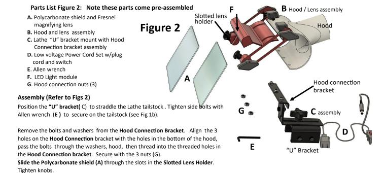
Slide the **Light Module** (F) between the knob shafts and under the washers at top of the **Hood.** Tighten the 2 top knobs to secure the light module. Note: Position the **LED light module (F)** by sliding it forward or back on top of the hood.
