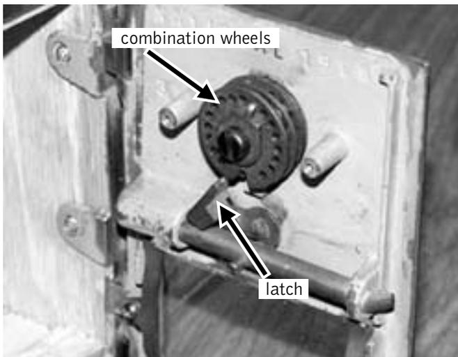
2. Loosen the large screw far enough that the washer with the 90 dog can be lifted up from its present position. Turn right or left and insert the 90 dog into another hole in the combination wheel. Tighten the large screw.
