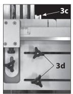
Make sure you attach and square your sled to the bandsaw table using the Adjustment Knobs (3d) and Adjustable T-Track (3a) Keep sled tight against the sides of the table.
