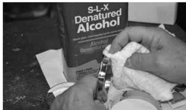
18) Wipe the inside of the bangle blank with denatured alcohol
