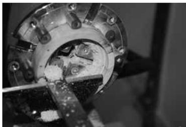
6) Stop the lathe frequently and use a Bracelet half (of the proper size) as a guide to see if it just fits inside. IMPORTANT – you want it to fit just a little loose so the glue will have something to adhere to when you glue the blank to the core. If it is too tight, when you glue it together, you will not have enough glue to make the pieces stick together.
