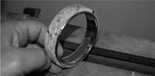
13) Mount the brass bushing core with your blank on a four jawed chuck to turn the outside diameter down to the brass bushing. You are using the metal brass bangle as a bushing to turn the blank down to the desired shape. You do not want to use your finished metal pieces because you will scratch them at this point.
