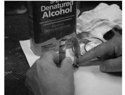
21) Use spring clamps to ensure a good bond between the finished metal core and blank. Allow it to dry for eight hours
