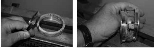
12) Place a piece of tape over the center of the brass metal core in a few places as shown to hold the core halves to the blank.
