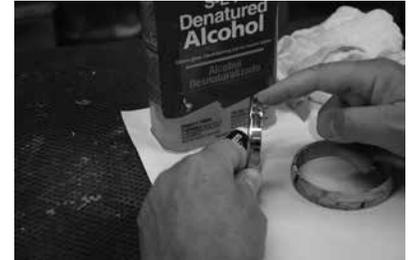
20) Apply a light amount of adhesive to the inside of the bangle blank.
