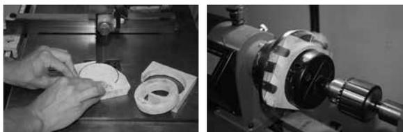
2) Drill the inside diameter with a 2 3/8" forstner bit. If drilling the inside hole on a drill press, it is recommended to drill the inside hole first (with a forstner bit) then cut the outside hole to 3-5/8" on a band saw.
