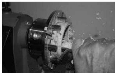
8) Once both sides fit properly, face off one side to get it squared up and start to reduce the width.
