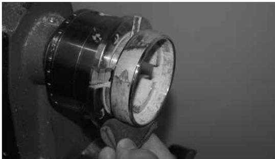
15) Apply a finish of your choice – A penetrating finishing oil (ie. similar to Mahoney’s, Odies, etc.) was used here for this blank. Buffing off the lathe will provide you with excellent results.
