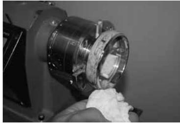
16) If you want to put a ca glue finish on the blank, remove the brass bushing core from the bangle blank and it is recommended that you make a jam chuck and apply the ca glue away from your four jaw chuck!
