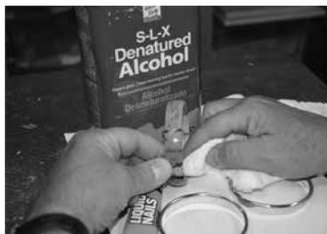
19) Apply a light amount of liquid nails (home version), this is flexible adhesive and will allow for movement without cracking) to the inside lip of both halves of the finished metal core. Other adhesives may work as well but should be flexible so they will not crack the wood after time as they dry out.
