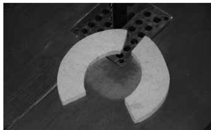
4) Mount a 4 Jaw Chuck (with #2 Jaws) on your lathe. Place the spacers behind the blank then open the jaws to tighten the blank onto the chuck and remove the spacers. DO NOT OVER TIGHTEN the blank – you will crack it or break it! If you have a set of mini jumbo jaws then you can place the blank inside the jaws.
