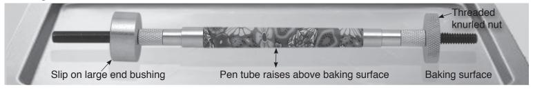
Assemble with large end bushings then place in oven to cure
