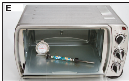
E Bake in oven at 275° for 30 minutes - allow to cool (OK to water cool)
