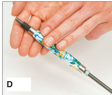
D Mount bushings and tube on mandrel - apply cane around tube. Mold to match bushings
