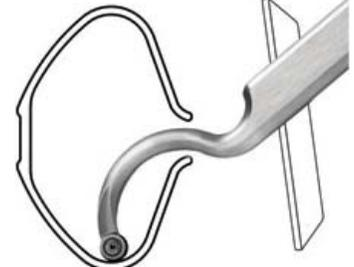
With a much greater curve, the #3 tool makes hollowing through the curve up to the lip of the opening an easy task.
