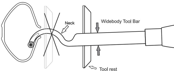
2. Set tool rest height so top of cutter is on center line.
