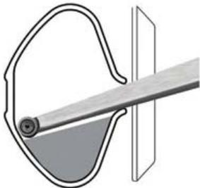
Grab this super versatile tool to begin all your hollow forms bowls & hollowing projects. and undercut where you can. Try it on bowls, coves and pens too. Works in holes down to 3/4" and reaches 4-1/2" (Mid-Size) to 8" (Pro) over the tool rest.
