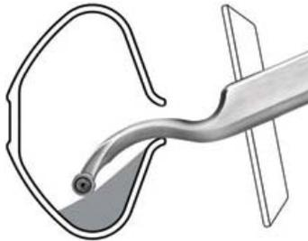
Choose this tool for clearing out the intermediate area in all your hollow forms and undercutting bowl rims. A must for working through small holes.
