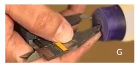
G. Mark the center of the Ring blank then use a caliper to clearly scribe the diameter on the blank that matches the OD of your ring.
