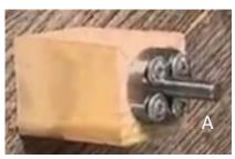
A. Use a piece of scrap wood for mounting your ring blank. Size about  $1-1/2 \times 2''$  long. Mark the center and use 4 screws to mount the Face Plate in the center
