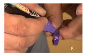
K. If using a transparent blank (i.e. many plastics) it will be necessary to paint the ring exterior a matching color
