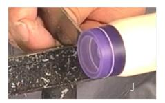
J. Measure the width of the ring with a caliper. Use the caliper to scribe a line on the blank with a parting tool to the exact width of the comfort ring. Part the ring exterior completely off the blank. Clean up any rough edges
