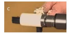
C. Use a roughing gouge to turn the scrap wood to about 1" round. Then D. Part the Face Square with a parting tool and flatten with a Spindel gouge to make a flat surface to the ring blank
