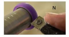
N. Turn and smooth the edges of the ring blank around the Ring core
