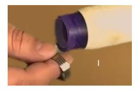
I. Continue to size the ID of the Ring Blank until the Comfort ring slides easily inside. Make sure there is sufficient depth to accept the ring width.
