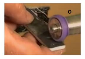
O. Sand the blank down the same as any other turning project. Start with 150 grit through 600/800 Aluminum oxide paper. Wet sand with the ultra fine sanding sticks for a polished finish. Wood rings can be sealed with CA glue.
