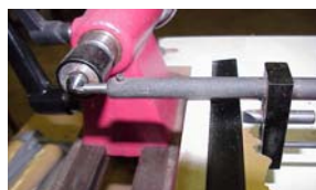
Fig 2 Aligning Duplicator with Lathe Headstock
