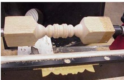
the balance of the spindle square as shown in figure 10. Mark and cut the square part of the spindle to be 1" square as
