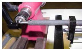
Fig. 3 Aligning Duplicator with tailstock end of Lathe
