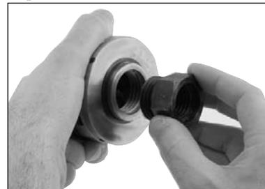
**Mounting the Chuck to Your Lathe**
