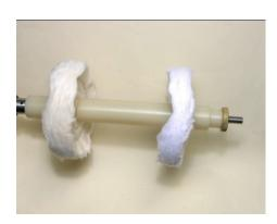
Next place the large 4" white spacer on the mandrel shaft followed by the 4" flannel (white) buff wheel, the remaining 2" white spacer with the tenon and the locking nut. Bring up tail stock to support buffing mandrel. The white wheel does **not** get rouge applied to it!
