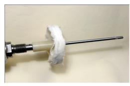
Insert the # 2 Morse Taper, 8mm mandrel into the head stock. Now, slide the 2" white plastic bushing onto the mandrel shaft followed by the 4" cotton (tan) wheel as shown. The tan wheel is the rouge applicator wheel.
