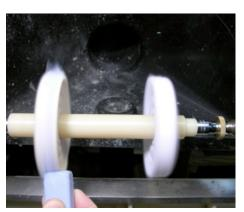
Apply a small amount of the blue polishing rouge to the cotton (tan) wheel. The cotton wheel should show slight traces of the blue plastic polish on the wheel. **ONLY** place the blue plastic finish on the cotton (tan) wheel. **DO NOT** place any of the blue plastic polish on the flannel (white) wheel! The flannel (white) wheel is the last step in the polishing process and should not have any blue polish on the wheel!
