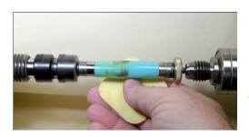
Use water to wet sand your acrylic pen blank as per your normal finishing methods. If you use a scratch remover, you may proceed to that step before removing your pen blank and mandrel from the headstock.
