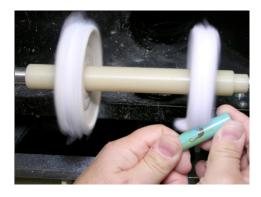
After you are finished with the cotton (tan) wheel, use two hands rotating the pen blank side to side and up & down to remove any hints of blue polish that might remain on the pen with the finishing flannel (white) wheel for approximately 10 seconds. Inspect your pen blank to ensure a glass finish with NO SCRATCHES!!!
