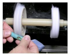
Lathe speed should be between 1,200 – 1,700 RPM.
