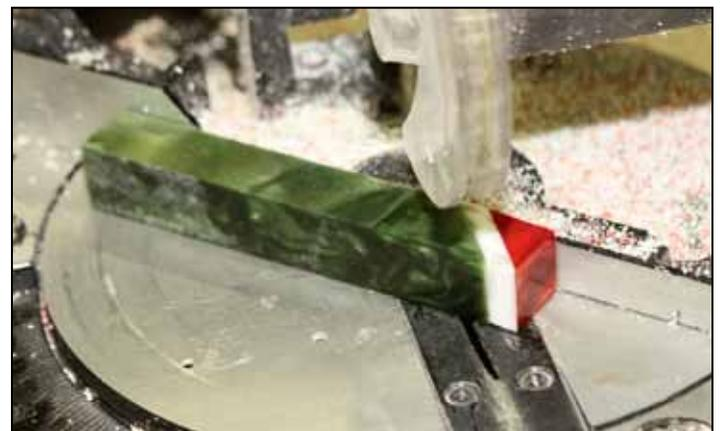
**Step 5 Cut your blank(s) to the tube length and square up the ends**
