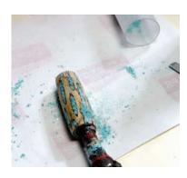
Step Fourteen: If you have any voids in the blank after turning it down, re-fill the area with the turquoise and return to the lathe to smooth it out.
