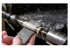
Step Fifteen: Sand the blank as you normally would to 800 grit and then use Abralon sanding pads (PKFINKIT2) to
