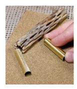
Step Two: Rough up the pen tubes so the glue will have a good bonding surface with the tube and the inside of the cactus.
