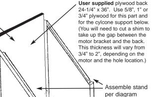
User supplied plywood cylone support: 24-1/4" x 24-1/4" with an 18-1/4" dia. hole. Locate the hole centered left to right. Depending on the thickness of the plywood, the location front to back varies from 3-7/8" between the hole & front edge of the base for Tempest, and 2-1/8" for the Tempest 2. (See note below)
