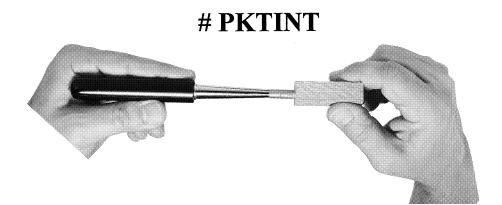
This tool can be used to aid in the insertion and gluing of pen tubes between 7 mm and 11 mm. Simply place the pen tube over the end of the tool and cover with your choice of glue. Be sure to cover the entire surface, leaving no bare spots. Slide the tube inside your pen blank with a twisting motion, while still on the tool. Slowly release the tool from the tube inside the blank, making sure the tube is centered. Allow your work to dry the prescribed time.
