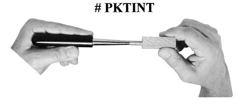
This tool can be used to aid in the insertion and gluing of pen tubes between 7 mm and 11 mm. Simply place the pen tube over the end of the tool and cover with your choice of glue. Be sure to cover the entire surface, leaving no bare spots. Slide the tube inside your pen blank with a twisting motion, while still on the tool. Slowly release the tool from the tube inside the blank, making sure the tube is centered. Allow your work to dry the prescribed time.
