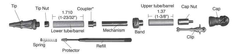
\*WARNING: Do not press directly on threads
