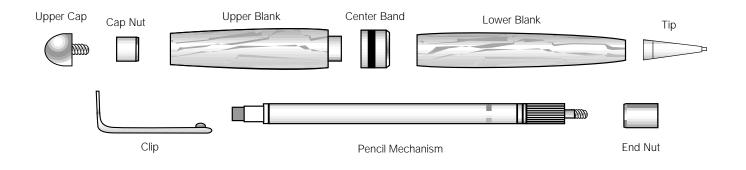
Cutting the Tenon - Keep the center band away from the upper blank. Make a pencil mark 7/32" from end. Use a parting tool to cut a 7/32" tenon down to the diameter of the bushing. Use the center band to test for a good fit over the tenon. Make sure you keep a sharp outside 90' corner on the tenon. Finish, varnish and wax both blanks.
