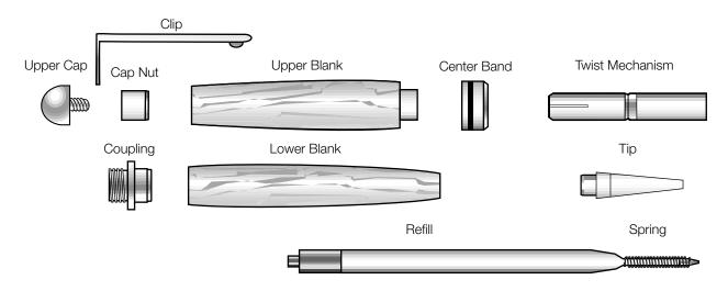
• Cutting the Tenon - Keep the center band away from the upper blank. Make a pencil mark 7/32" from end. Use a parting tool to cut a 7/32" tenon down to the diameter of the bushing. Use the center band to test for a good fit over the tenon. Make sure you keep a sharp outside 90° corner on the tenon. Finish, varnish and wax both blanks.
