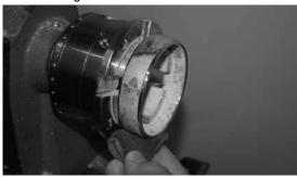
15) Apply a finish of your choice – A penetrating finishing oil (ie. similar to Mahoney's, Odies, etc.) was used here for this blank. Buffing off the lathe will provide you with excellent results.
