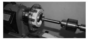
3) Make a set of spacers from a piece of 1/4" plywood or some other scrape wood as shown.
