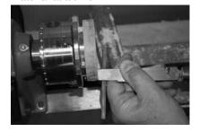
**10)** Stop the lathe and check it frequently until the bangle blank just fits inside the two halves as shown without having any gaps in the metal core.
