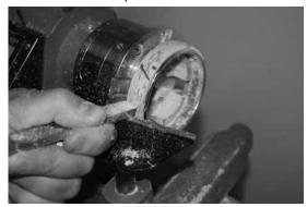
**14)** Once you have the desired shape to your blank, sand it on the brass bushing core and then use sandpaper (Abralon pads recommended) to finish sanding the blank.
