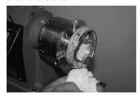
16) If you want to put a ca glue finish on the blank, remove the brass bushing core from the bangle blank and it is recommended that you make a jam chuck and apply the ca glue away from your four jaw chuck!
