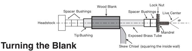
Note: Before turning the blank the inside wall of the blank needs to be trimmed square on the lathe.
