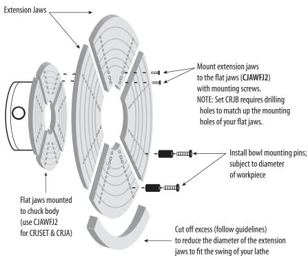
Required: PSI CJAWFJ2 Jumbo Jaws installed on your chuck
