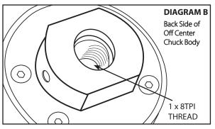
The CSC600 Off Center Chuck is like no other tool you currently own. Check the Parts List (Diagram A). For working on pieces that are not pens or bottle stoppers, the CSC600 chuck body is screwed onto the lathe headstock's 1x8tpi spindle and then a scroll chuck is threaded to it (face). The material your are turning is mounted onto the scroll chuck. The amount of degrees off center you cut is determined by the number of turns applied to the cross screw.
